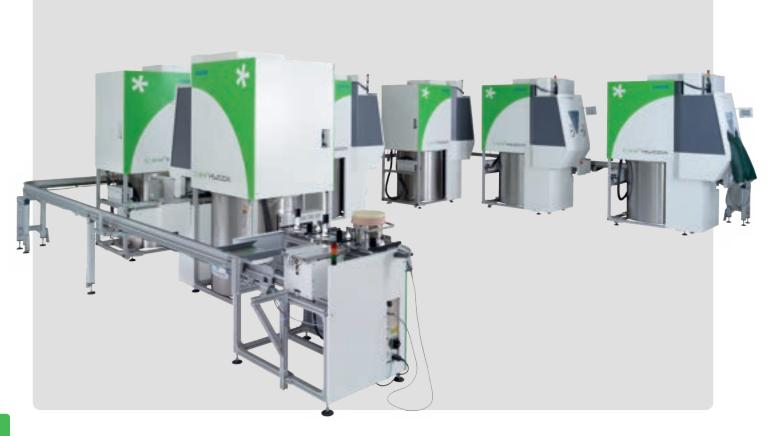
Connection of several ASKION C-line<sup>®</sup> hermetic storages to one fully automated biobank by using the external automation (rail system with shuttle and transfer station)
