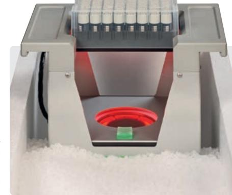
ColdEye<sup>+</sup> half submerged in dry ice
