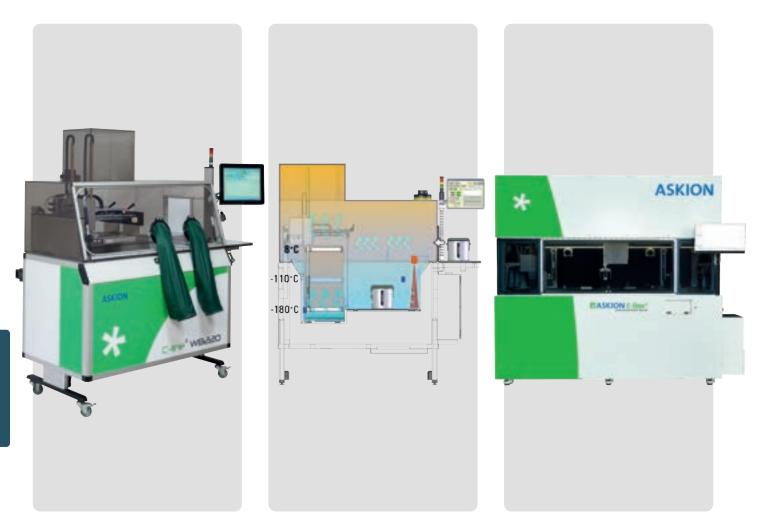
ASKION C-line® work bench (left) and transverse section of a ASKION C-line® work bench with temperature gradient (middle) and ASKION C-line® automated work bench (right)
