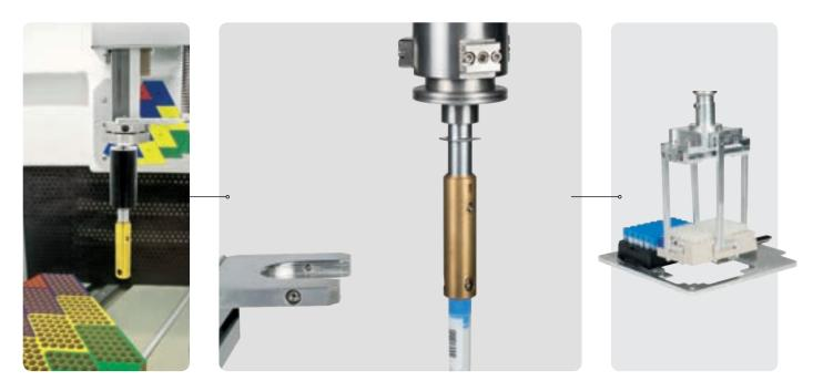
Pick-and-Place-robot above a tray at an ambient temperature below -100°C (left), gripper changing system of HS200 M/L with single gripped sample (middle) and SBS rack gripper (right)
