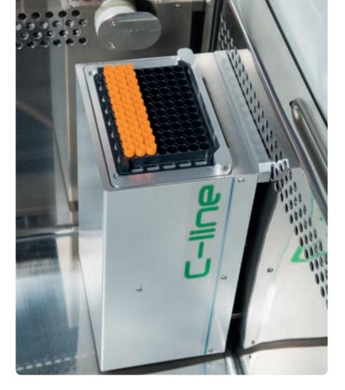
ColdEye installed inside ASKION C-line® work bench to identify samples below -100°C
