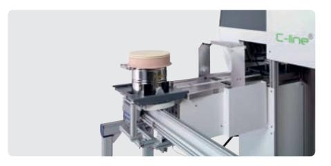
Shuttle with transport container waiting in front of the connecting station to transfer samples into the HS200
